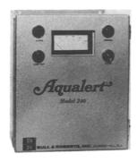
• Bull & Roberts' new Aqualert 240 oil contamination monitor can detect oil concentrations down to 10 parts per million. The device can be used by edible oil processors to facilitate recycling of condensed steam. The continuously operating device automatically compensates for varying turbidity, constantly measuring visible and ultraviolet light spectrums through the sample steam. Information: Bull & Roberts Inc., 785 Central Ave., Murray Hill, NJ 97974.
